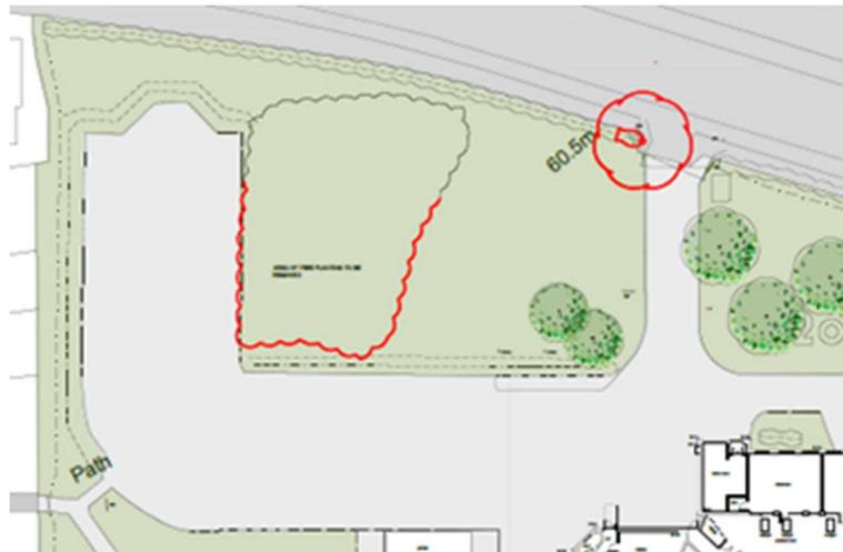
The below is the new final layout where you can see the entrance widened out and the additional car park adding in. The trees and hedge are removed to relocate the splay lines on the road to ensure it is easier to get in and out of the school. A new hedge will be planted back with a new fence. The trees that are removed are classed as low ecological value by the qualified ecologist who did the report for planning and we will also replace these plus more when we get to November later in the year.
